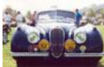
Bill Rooklidge's 1953 Blue XK120. Note the louvers on this one...just like Clark Gable's car. Jag put louvers on some of these cars sent to CA and AZ to dissapate engine heat in hot climates.
