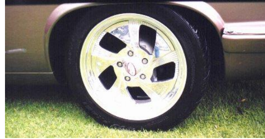
JERRY HATTO'S 1985 XJS WITH BOYD CODDINGTON 17 INCH POLISHED BILLET WHEEL LS HOLDING 245 45'S IN THE BACK AND 235 45'S IN FRONT
